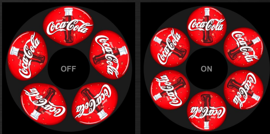
Visual Poi MAXI with image warping function disabled (left) and enabled (right)
