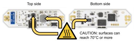
Note: FT2 chip contains thermal protection - if the temperature reaches 100°C, the chip will turn off to protect itself.
