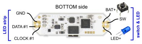
Connect a LED diode (forward voltage: 1.7-3.3V) between the **LED+** and any **GND** pad to get an external battery charging indication.
