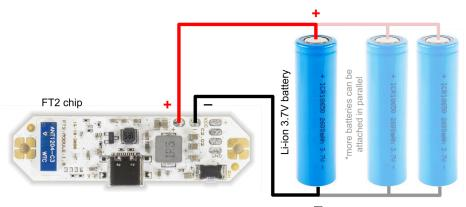
Caution: supplying voltage higher than 5V or reversing the polarity of the battery will damage the FT2 chip!
