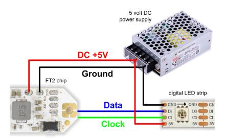
Note: In this configuration the voltage converter is not used, so it doesn't matter if it is bypassed or not.
