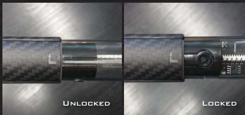
Visual Poi alignment and the locked position
