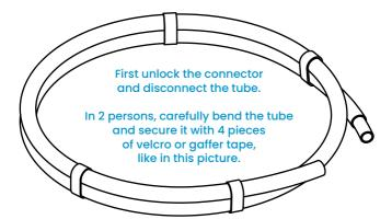
Do not lock the connector into a fully enclosed coil.
